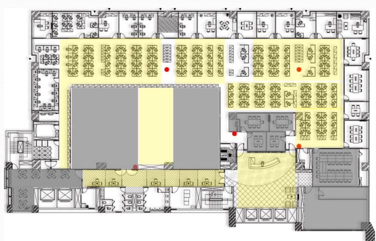
This figure shows the digital map of a office lighting system. The system is displaying lights with different color indicating their on/off status. You can also click on specific area of the map to turn lights on/off. You can replace traditional switch by running our system on a touch-screen tablet. You can also setup customized schedule to turn lights on/off at specific time automatically.
