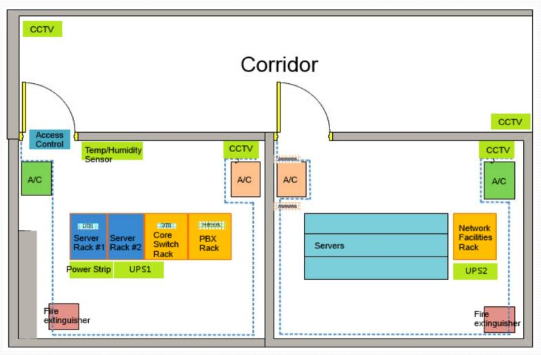
This figure shows the digital map of a monitored server room. When events occurs, corresponding icons start blinking and alarming, and related CCTV video will be played on system. Email or mobile SMS can also
