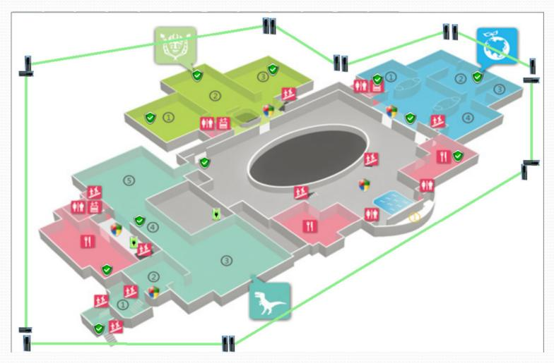
This figure shows the digital map of a monitored environment. When events occurs, corresponding icons start blinking and alarming. Email or mobile SMS can also be configured for receiving notification.
