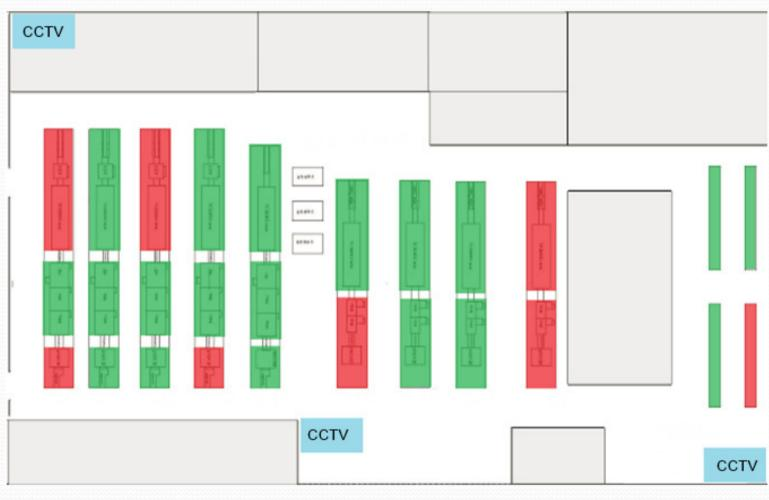
This figure shows the digital map of a manufacture workshop. The system is displaying equipments with different color automatically and periodically by calculating it's utilization rate on the fly. User can watch CCTV video on the system to catch up with real time status.
